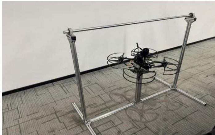
Figure 3. Attitude loop PID tuning.
